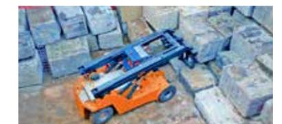
**ML5012R** is the world's smallest machine in its lifting capacity range of 50 tons. Horizontal boom structure and compact size enable it to handle heavy loads in confined spaces.
