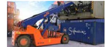
**ML1612R & ML1812R** is the only telehandler in the lifting capacity range of 16 tons, which can be operated inside containers.
