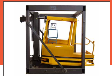
Strong, all-steel cab structure (fully FOPS and ROPS tested) ensures maximum driver protection
