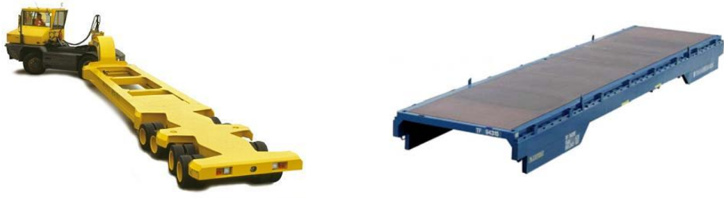
Figure 2. Terminal tractor, translifter and a cassette
